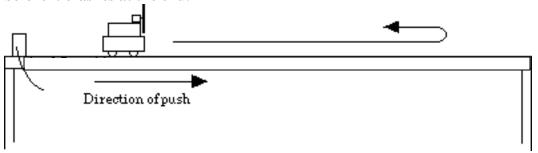
25. **Pre-Lab**: For each part of the motion after you release the cart—*away from the detector*, *at the turning point, and toward the detector*—predict in the table that follows whether the velocity and acceleration will be positive, zero or negative.
