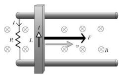
If there is a current *I* flowing upward through the bar, the magnetic force on it is *ILB* to the left on it. Someone or something must apply the same size force to the right on the bar to keep it moving at a constant speed. Of course, once we've got a *current* flowing up the wire, there's a force exerted on it back to the left to the tune of
