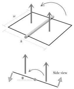
The emf is largest when the angle  $\theta$  is 90°, because the wires are moving the fastest in the direction perpendicular to the magnetic field. The size of the emf on the left wire depends on the component of the velocity perpendicular to the magnetic field:
