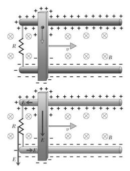
Then the *emf* separates charge and that charge separation drives current through the resistor.
