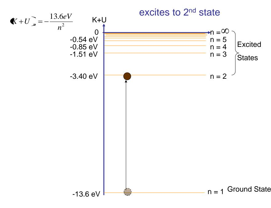
Hydrogen Excitation: 3<sup>rd</sup> Looses Energy by photon emission,
