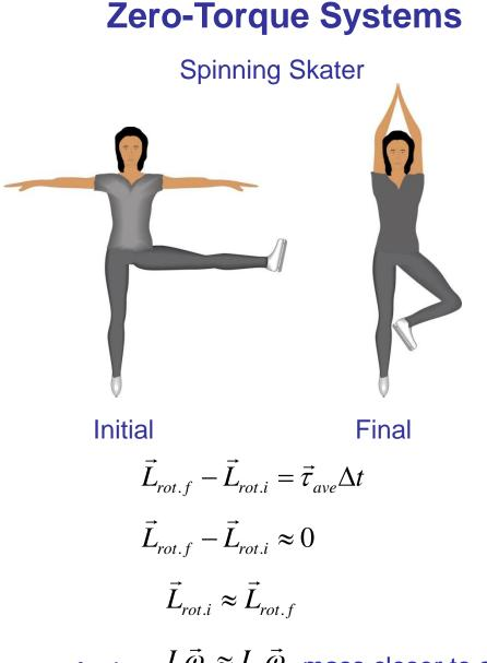
mass farther $I_i \vec{\omega}_i \approx I_f \vec{\omega}_f$  mass closer to axis:from axis: $I_i$  larger $\omega_i$  smaller $\omega_i$  larger
