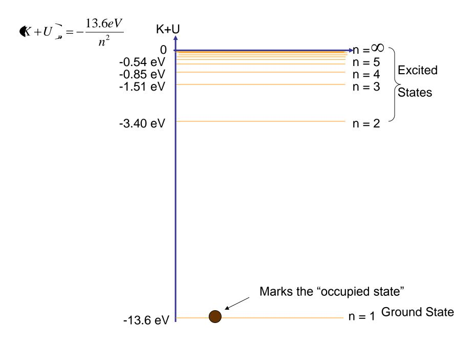
Hydrogen Excitation: 2<sup>nd</sup> Adsorbs energy from Collision
