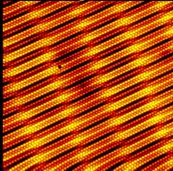
A 180×190 Å<sup>2</sup> Image of the Pt(001)-hex reconstructed surface taken with a custom Scanning Tunneling Microscope at Aarhus University's Scanning Probe Microscopy lab. The dark spot near the center is a single, missing atom.
